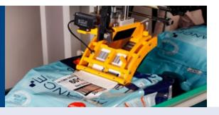
The MD-1500 is Zetes' decorative labelling machine. It can be operated in label only mode and print & apply mode as needed. Designed and built in-house by Zetes, the MD-1500 is an economic solution for your basic packaging execution needs.
